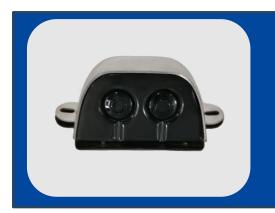
Using ZETA based wireless supersonic sensor to detect if a parking place is occupied by vehicles.
